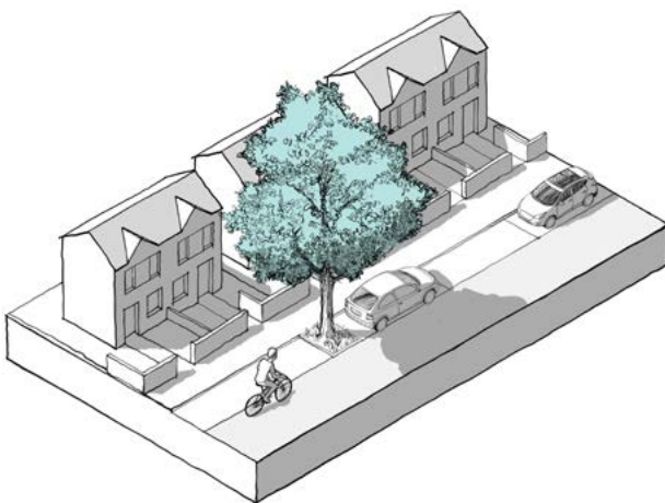
Figure 224: Street tree planting incorporated within the parking area to avoid disrupting the pavement or carriageway as set out in the National Model Design Code.
